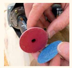
**Replacing Discs.** The high pressure glue on the back of the discs is formulated so the discs can be cycled through grades.
