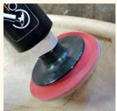
Tight Corners. The flexible pad follows contours all the way into the tightest of crevices, perfect for spot sanding.
