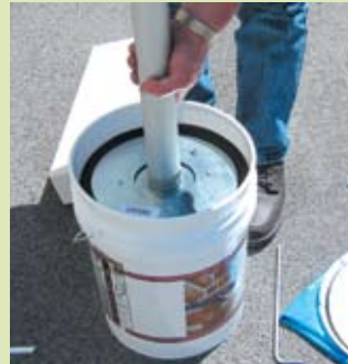
Remove the cap and cone tip from the gun barrel and push the end of the barrel onto the hole
