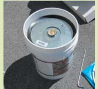
Place the follow plate on top of the chinking pail
