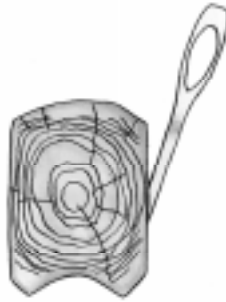
1900 Model Reverse Scissors Sharpening. For squaring of logs or for the planing of log walls. “Carving Broad Axe”
