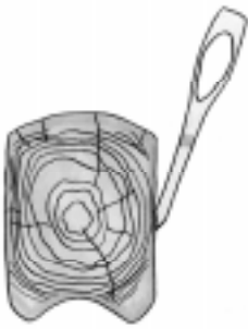
1900 Model (Most Common) Double-sided Sharpening for all types of hewing of timber and corner chopping “Chopping Broad Axe”
